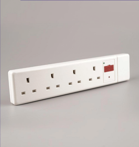
Fused 13A, Rewireable 4 Gang Extension Socket with Neon Indicator + 2M BS Cable (3Cx1.25) & Plugtop
