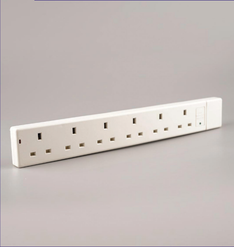
Unfused 13A Rewireable 6 Gang Socket with Neon Indicator + Surge Protection + 2M BS Cable (3Cx1.25) & Plugtop
