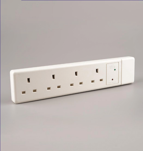
Unfused 13A, Rewireable 4 Gang Extension Socket with Neon Indicator + Surge Protection + 2M BS Cable (3Cx1.25) & Plugtop
